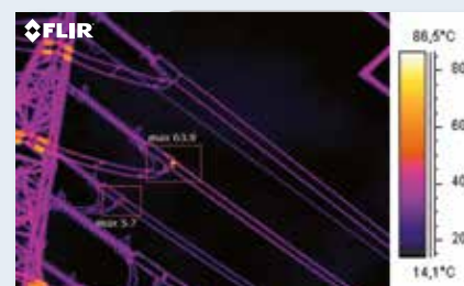
Image taken with 640 x 480 pixels resolution and <45mK thermal sensitivity. Notice how the hot spot now is clearly visible and that the increased number of pixels will result in an even more accurate temperature reading in the hot spot. It is now clear that there is a problem in the power line.
