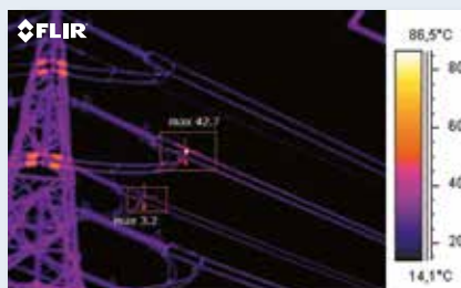
Image taken with 320 x 240 pixels resolution and 50mK thermal sensitivity. Please note how the increased number of pixels will result in a more accurate temperature reading in the hot spot.
